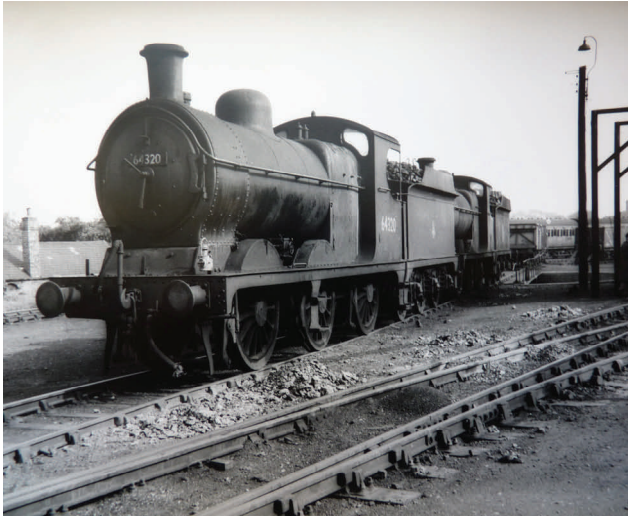
The two locomotives in the photograph are J11 engines at Louth shed, designed by Robinson for the Great Central Railway in 1901. They acquired the name 'Pom-Poms' due to the similarity of their exhaust noise to that of the 'Pom-Pom' quick firing gun used in the South African War
